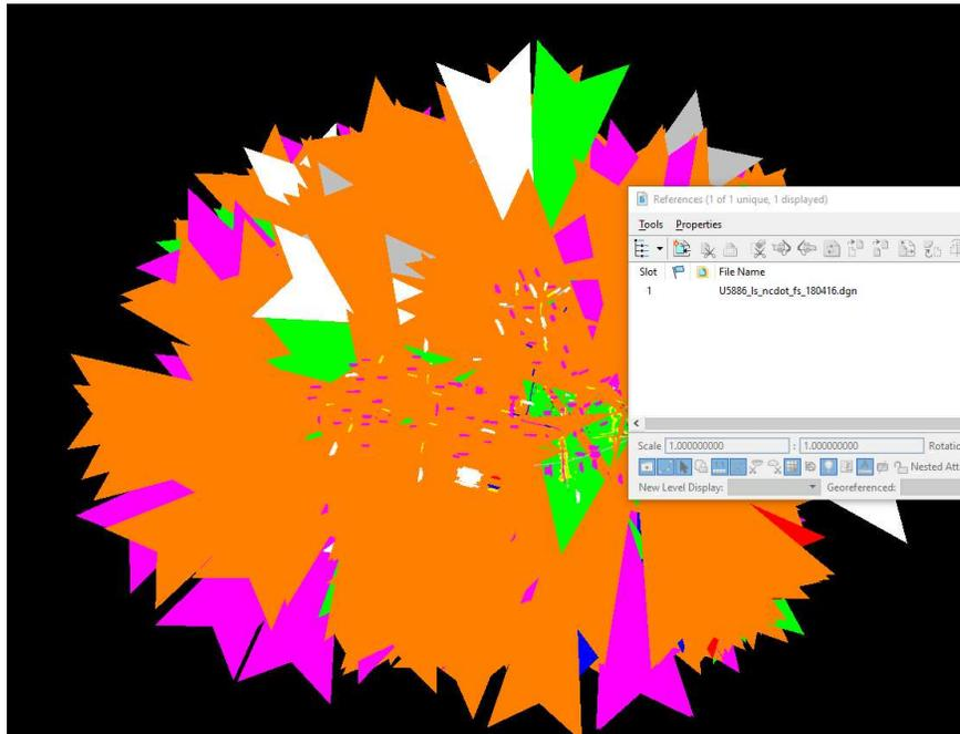
*Figure 22 - First indication of scaling errors.*
